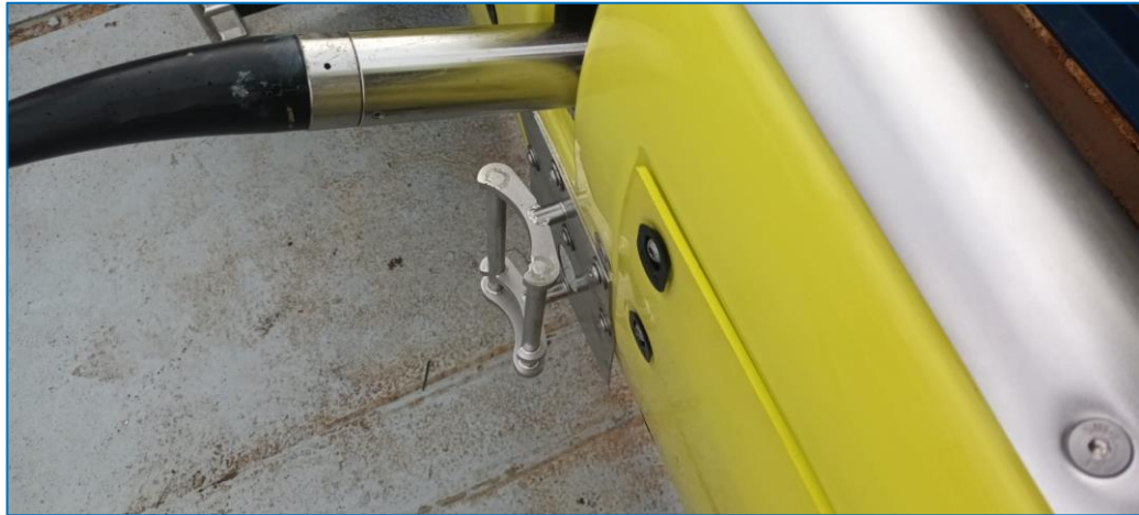
Figure 1.1 USBL transponder mounting position on the ScanFish body
